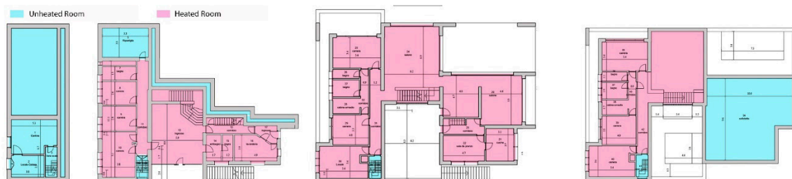
Figure 3. View of thermal distribution.
