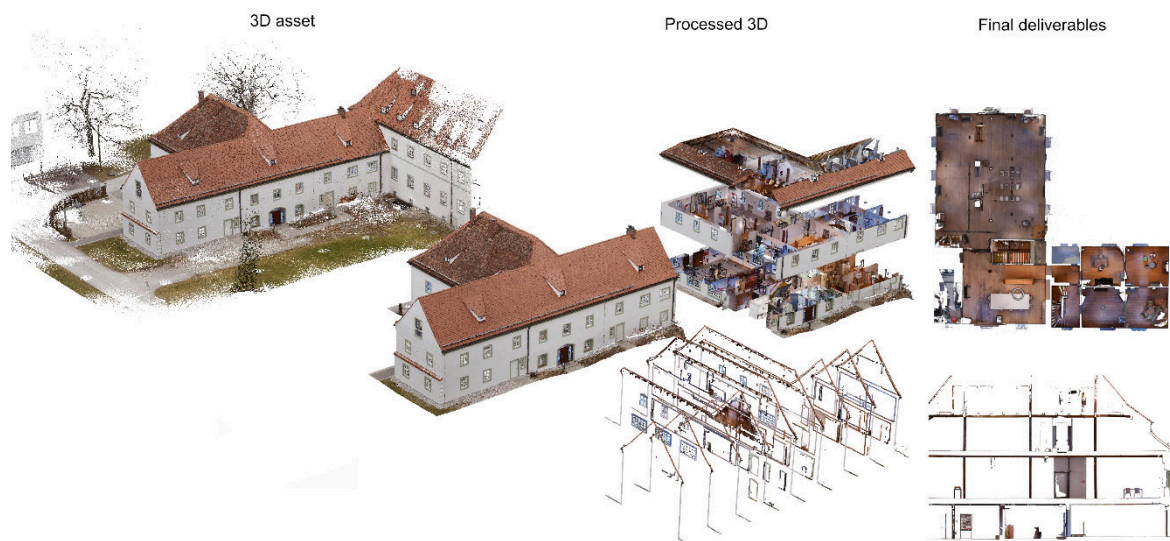
Figure 4. An illustration of data processing: Merged point cloud of the envelope and the interior spaces processed into slices and then key orthoviews (images)
