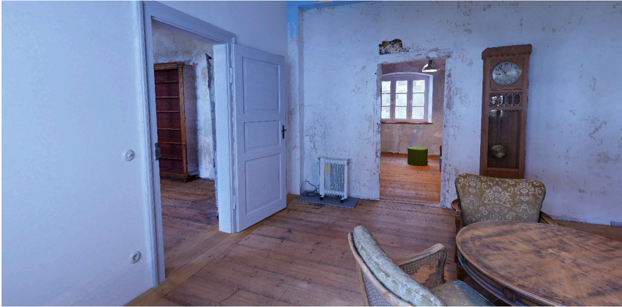
Figure 7. Combining TLS and photos to maximize both geometrical accuracy and textural quality (illustration: mesh from combined photos and laser scans)
