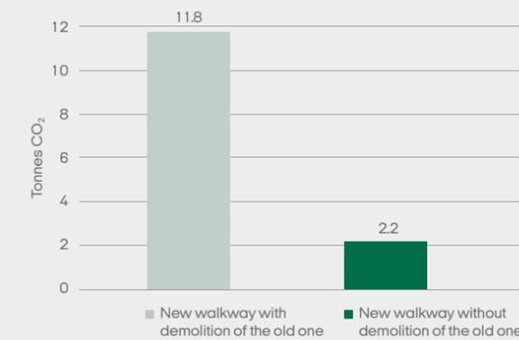
Graph illustrating the issue of "double demolition": Carbon impact of replacing the walkway around Dyrehave Mill, including both demolition of the old balcony and the new walkway, and an alternative LCA including only the new walkway.
