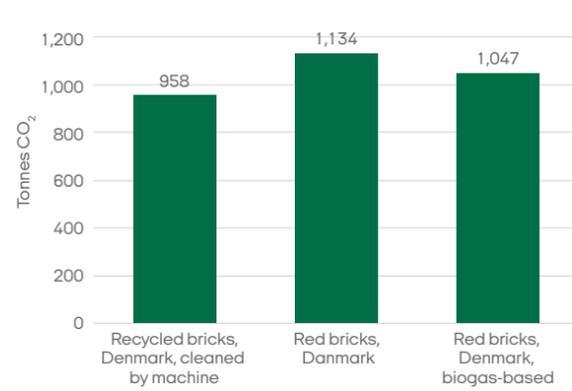
Total CO<sub>2</sub> emissions for the transformation of the farm buildings, as calculated [with recycled bricks], and what they would have been had new bricks been used.
