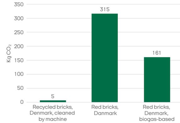
The difference between CO<sub>2</sub> emissions for one tonne of bricks: recycled bricks as used at Hinds-gavl and various possible new bricks [including manufacture, disposal and waste treatment].
