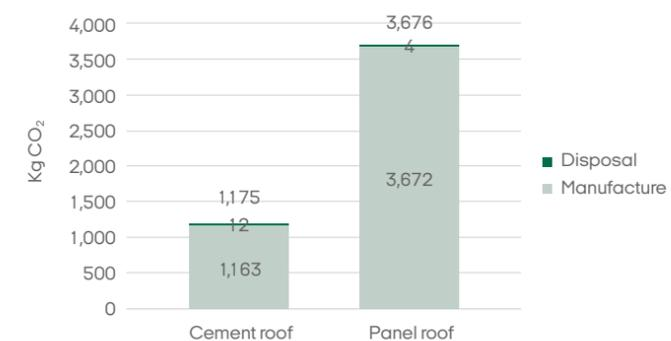
↑ CO<sub>2</sub> emissions for the 118-square-metre tile roof on the farmhouse and 268-square-metre panel roof on the other buildings. Only the two materials are included here, and not the underlying roof structure with the rafters, roofing felt, etc.
