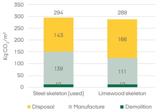
Total CO<sub>2</sub> emissions for restoration of the barn at Højergård using the current girdle and an alternative to stiffen the building.
