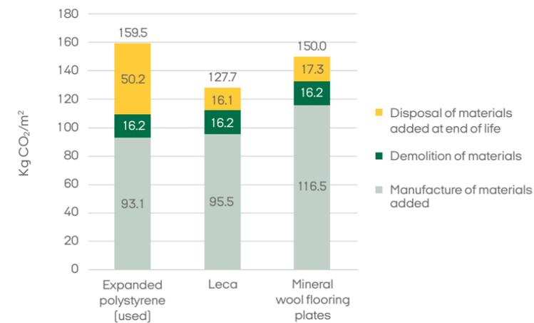
↑ Bottom: Carbon emissions per square metre of the total restoration of the Roman House and future disposal using different insulation materials in the flooring, broken down by phases. Polystyrene is “best” in the manufacture phase but loses in the long term with disposal, particularly if ongoing heating of the house is not included.
