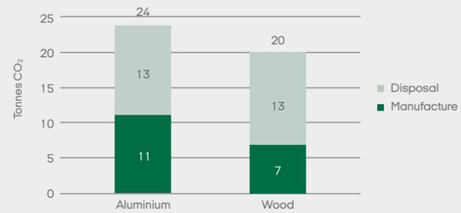
↑ CO<sub>2</sub>-emissions of the full restoration of Poul Henningsen's house using aluminium window frames compared with wood window frames. This graph shows the difference between aluminium-framed secondary glazing and, as another option, wood frames.
