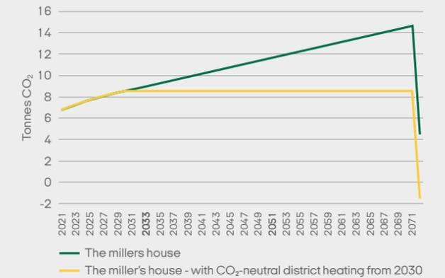
These two graphs show CO<sub>2</sub> savings from insulating the farmhouse and the garage building using wood fibre. Insulation of the garage building will continue to be a CO<sub>2</sub> benefit, while the miller's house will end as a cost, if CO<sub>2</sub>-neutral district heating is fitted in 2030, as there was a certain amount of loft insulation previously.
