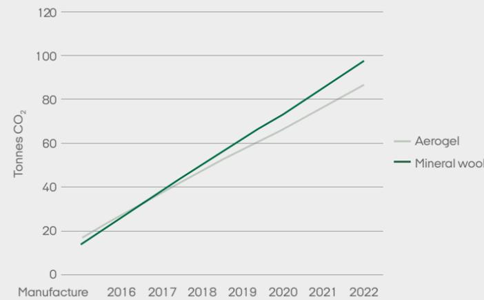
↑ CO<sub>2</sub>-emissions using 2 cm aerogel vs. 2 cm mineral wool Using aerogel has paid off in terms of CO<sub>2</sub> around two year after restoration of Poul Henningsen's house, because the house is better insulated and therefore emits less CO<sub>2</sub> for heating.
