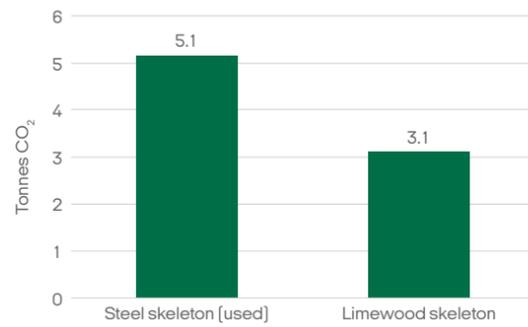
CO<sub>2</sub> impact from fitting the steel skeleton in the barn at Højergård to preserve the old walls, compared with a 50% larger timber skeleton.
